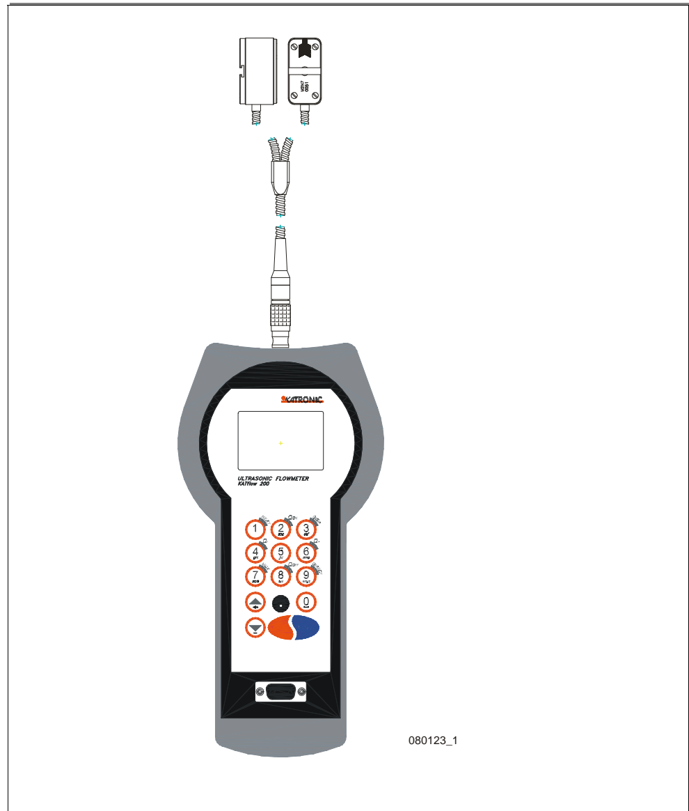
Drawing 3: Electrical interconnection diagram KATflow 200
